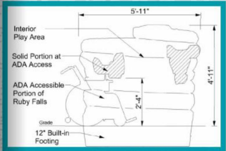
**Ruby falls is a sand and water table that is push button activated, resulting in a fast flowing creek through the ridges and dams of sand. A specially designed area allows wheelchair access, allowing anyone to join in the fun. The wheelchair accessible section should be used with unitary safety surfacing.**
